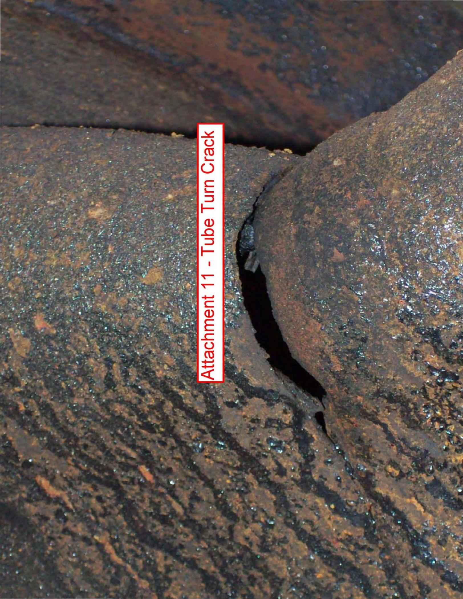
A close-up photograph of a rusted metal pipe joint. The metal is heavily corroded, showing a dark brown, pitted surface. A significant crack is visible in the pipe wall, extending from the joint area. The crack is dark and appears to be a through-hole. The surrounding metal is also heavily rusted and textured.
